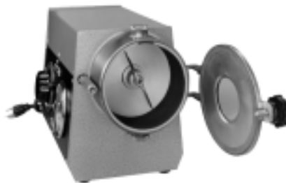
Fig. 1—Accelerotor fitted with abrasive liner over foam rubber cushion and with 114 mm (4.5 in.) S-shape rotor.
